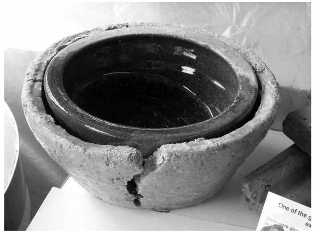
Fig. 4 A pot after firing with glassy rim (front) and deposits formed from reactions with fuel ash (back) (Courtesy of J. Bayley).
