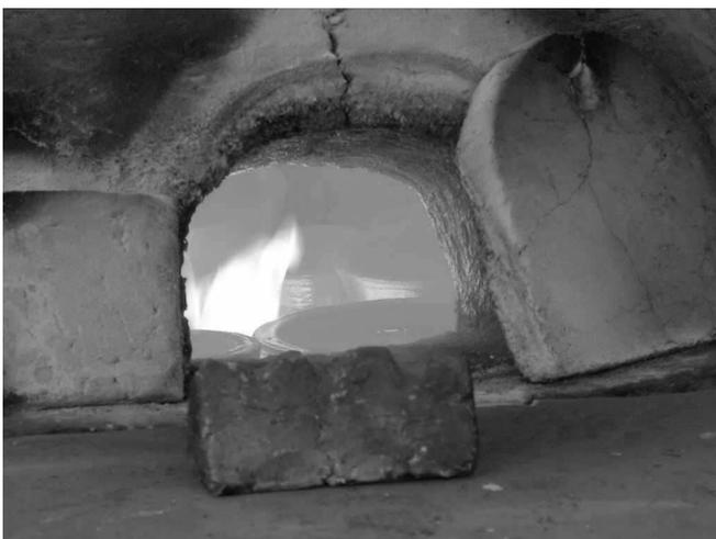
Fig. 3 View of pots in the furnace during firing (Courtesy of J. Bayley).
